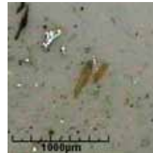
Second largest nonmetallic particle 387 µm x 76 µm
