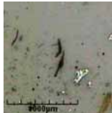
Largest nonmetallic particle 542 µm x 121 µm
