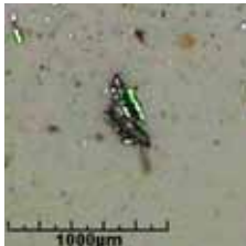
Largest metallic particle 660 µm x 229 µm
