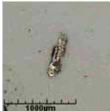
Second largest metallic particle 644 µm x 177 µm
