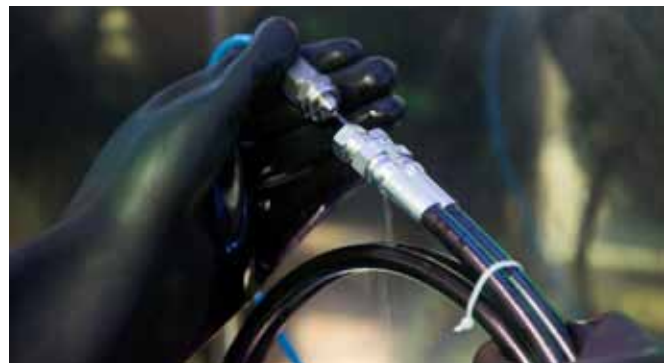
Pressure rinsing of hydraulic hose
