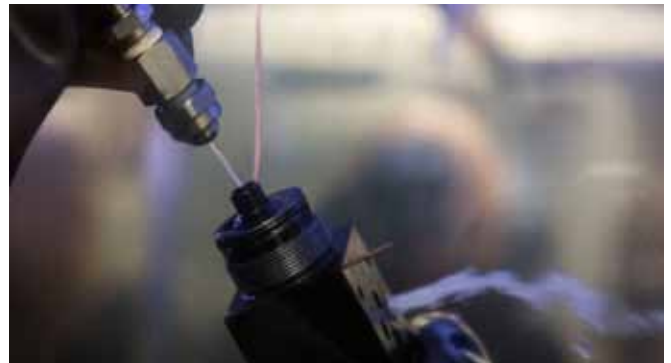
Pressure rinsing of manifold block
